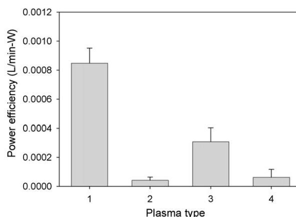
Note: <sup>1</sup>Gliding Arc Plasma (this experiment), <sup>2</sup>Plate DBD (ref. 30), <sup>3</sup>Tube DBD (ref. 10), <sup>4</sup>RF plasma (ref. 31)
