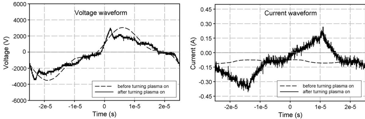
Fig. 2. Applied voltage and current waveform.
