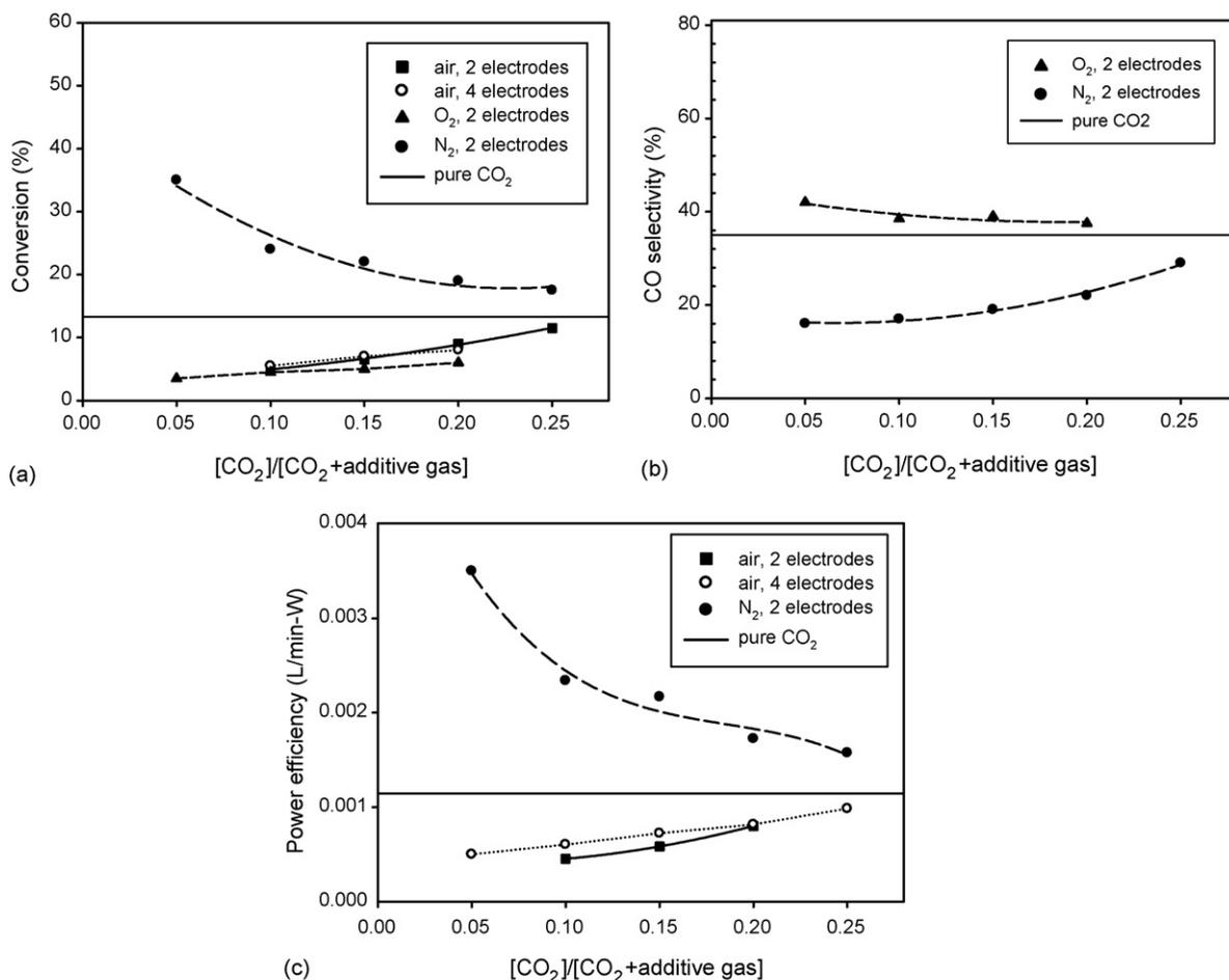
Note: 2 electrodes mean 1 anode and 1 cathode, 4 electrodes mean 2 anodes and 2 cathodes
