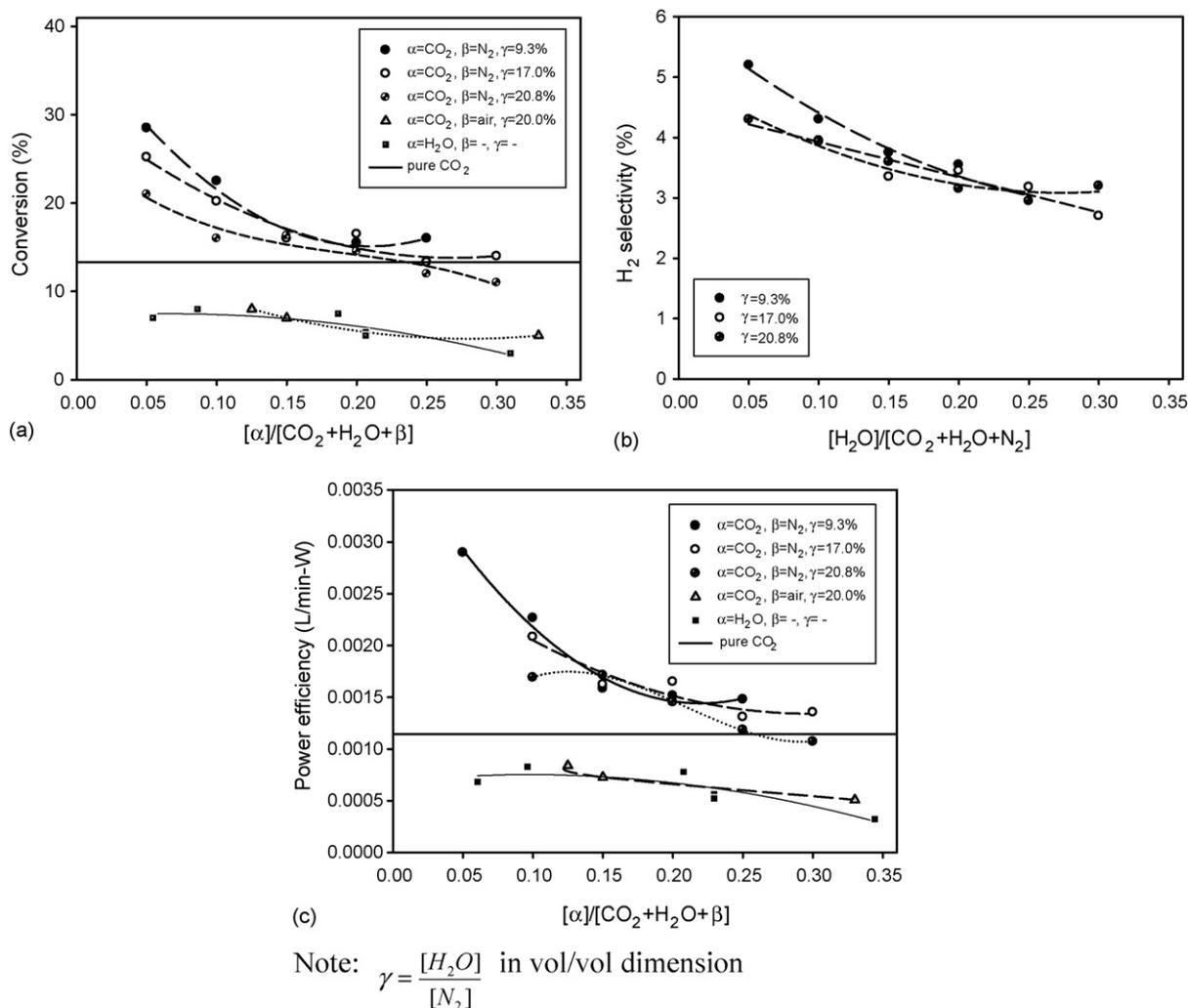
Fig. 5. Effects of water vapor on (a) CO<sub>2</sub> conversion, (b) H<sub>2</sub> production, and (c) power efficiency. The experiment was conducted at fixed flow rate of 2 L/min and frequency of 20 kHz.
