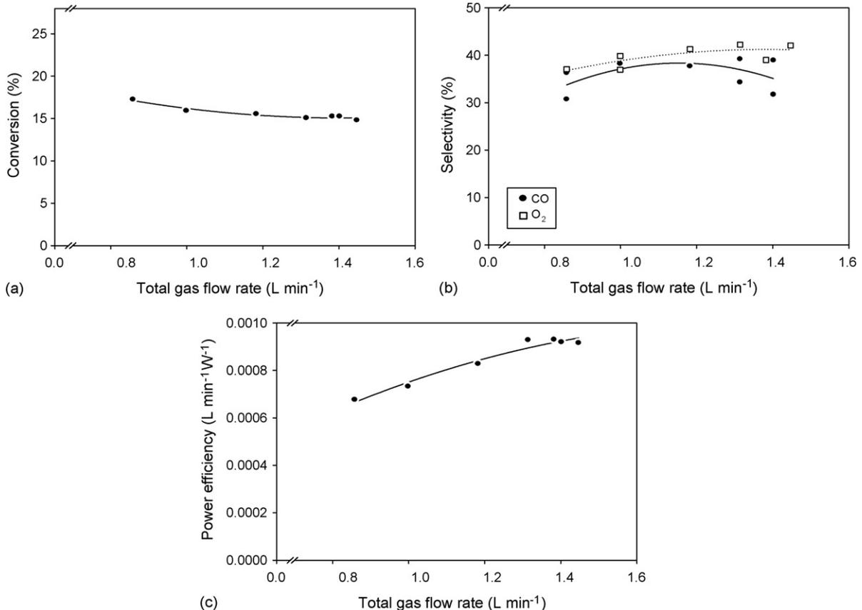
Fig. 3. Effects of total gas flow rate on (a) CO<sub>2</sub> conversion, (b) product selectivity, and (c) power efficiency. The experiment was conducted at pure CO<sub>2</sub> condition and fixed frequency of 20 kHz.
